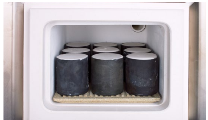
Flexibility: 9 x #3, 4 x #6, 3 x #9 casting rings
